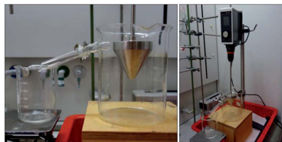
Fig. 1 Separation beaker with a stirring device and displacement cylinder.
